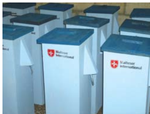
Bio-sand filters completed with community for pilot project, Sri Lanka
